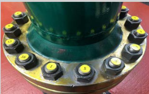
They are designed to be attached anywhere around the flange or joint or to the top of the bolt itself on larger applications, They are so slim that they can be stacked on top of each other. This enables the user to control multiple passes during bolt tightening operations. As each bolt is tightened in the correct sequence the coloured button is removed signifying that part of the operation is complete, making it extremely easy for the operator to keep on top of where they are in the process.
